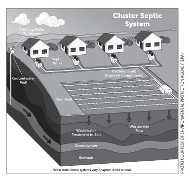
The downtown sewer system will be similar to the cluster system shown here. The difference is that the waste water from onsite septic tanks will be conveyed to a secondary treatment facility and drain field at Bernard Memorial Park.
